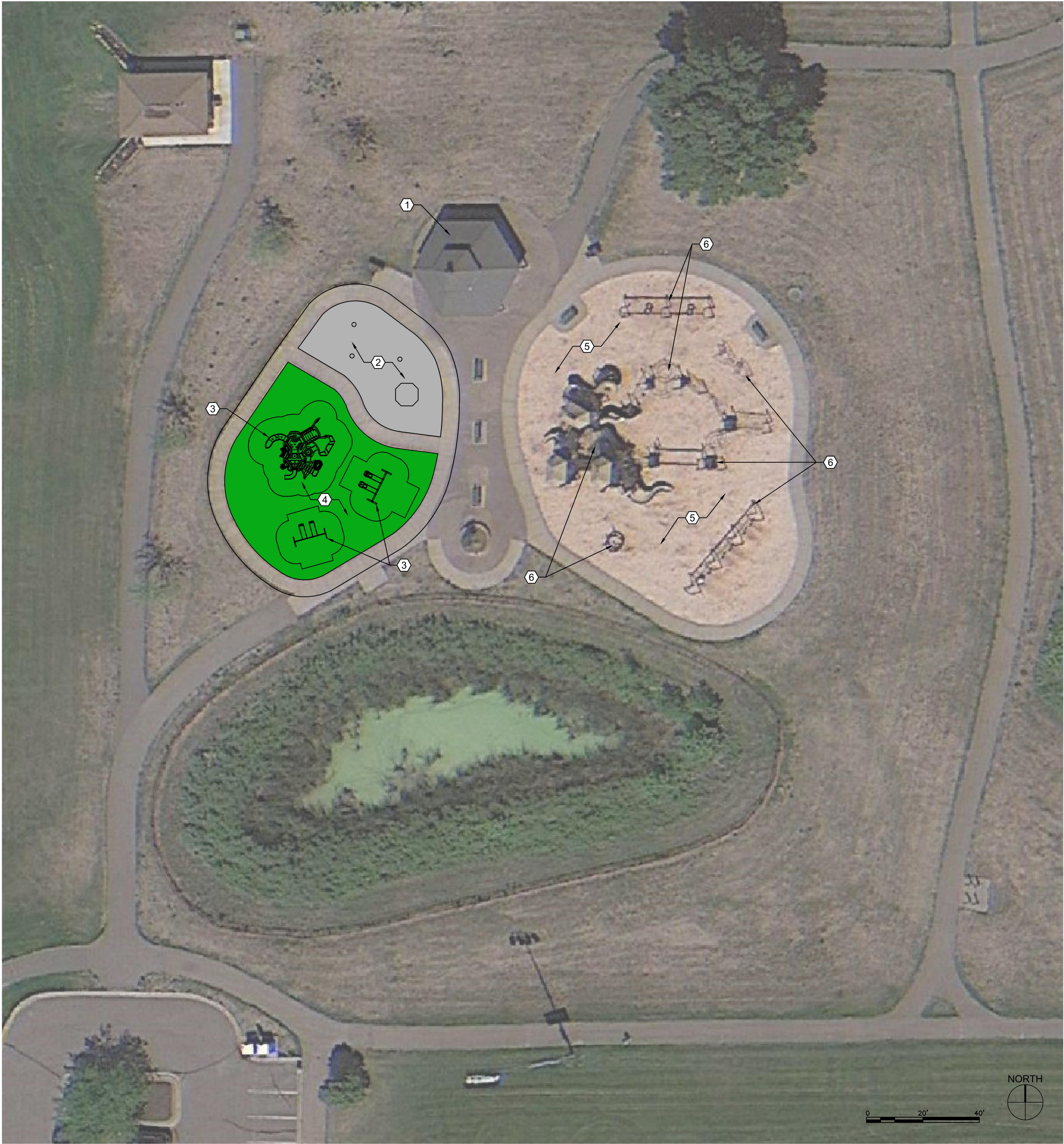
① REFURBISH EXISTING SHELTER 1. SANDBLAST EXISTING STEEL MEMBERS 2. REPAINT STEEL MEMBERS
